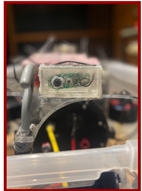
Figure 9 (top left), Figure 10 (bottom left), & Figure 11 (right): Cameras facing the claw, the front end of the ROV, and the back of the ROV coated in thick layers of epoxy resin. (Photos taken by Anton Chen via iPhone)
