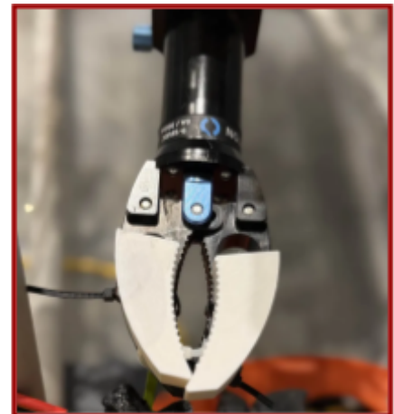
Figure 7: Blue Robotics Newton Subsea Gripper With 3D-printed improvements
