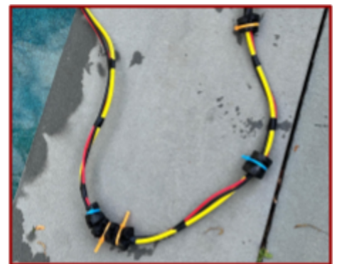
Figure 12: Our negatively buoyant tether. (Photo taken by Ilaria Luna, via iPhone)
