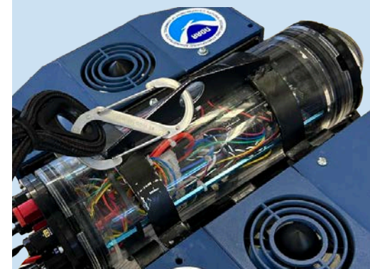
Strain reliefs at both ends of the tether. We use the carbine clips for quick removal in case of emergency
