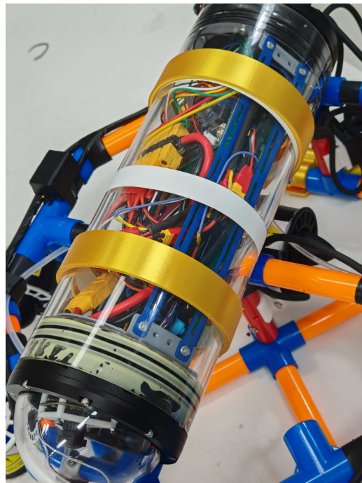
FIGURE 39: THE FASTENERS OF THE 3D-PRINTED SEALED CABIN
