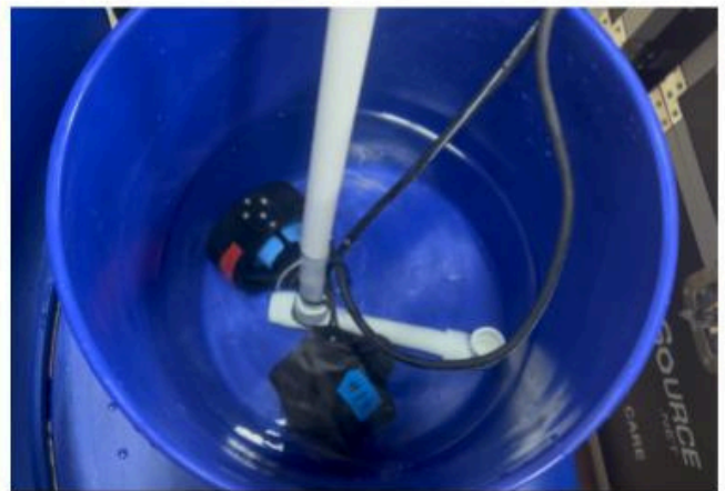
Figure 3: Submerged thruster test to determine power usage
