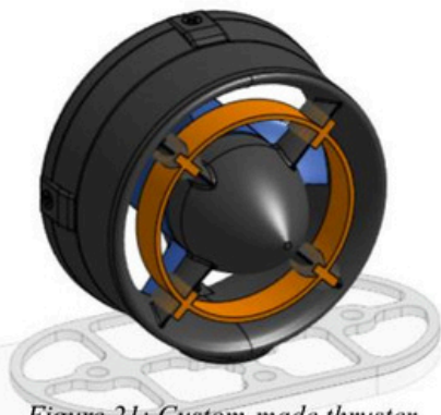
Figure 21: Custom-made thruster guard in orange
