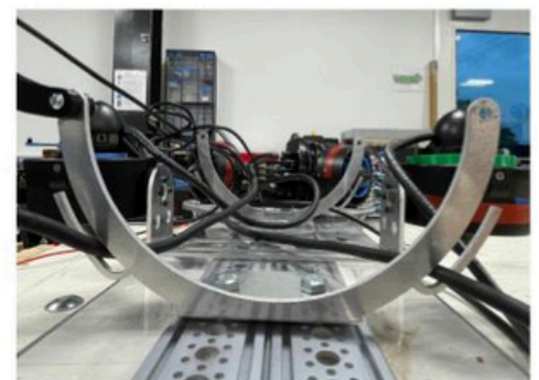
Figure 10: Hub clamps with cable management prongs on sides
