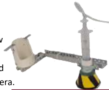
E-DNA Syringe with Funnel Closeup Photo Credit: N Scott
