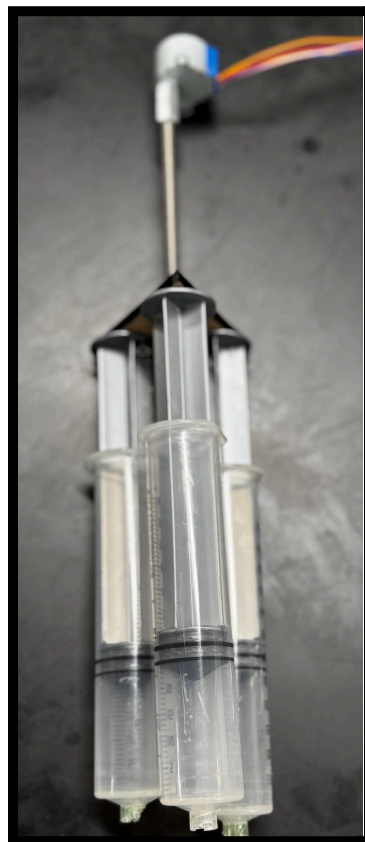
Three syringe dynamic machine attached to a stepper motor connected to the Raspberry-pi control system
