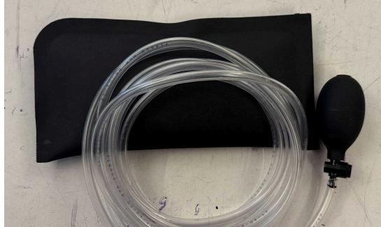
Figure 12: Inflatable jack: A repurposed inflatable jack has high durability and amount of air can be adjusted.
