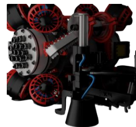
Figure 37 Water sampler mechanism
