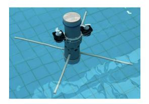
Part 1 is the Airtight Electronic Housing Part 2 is the Weighted Support Structure
