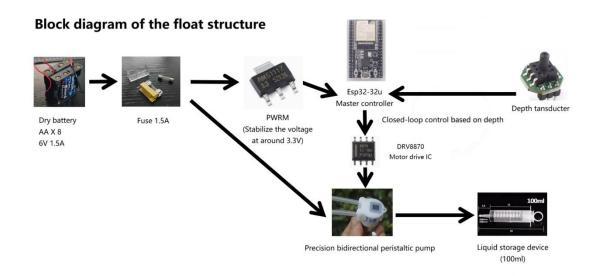
The basic structure of the underwater float system is divided into the following modules:
