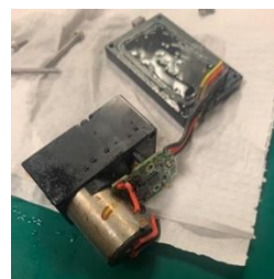
Figure 3.2.1. Waterproof Servo Motor Leaking Water
