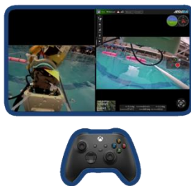
Figure 3.7.2 Dual Camera Control System
