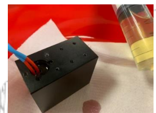
Figure 3.2.2 DIY Waterproofing by Adding Oil to the Servo
