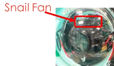
Figure 3.3.2 Snail Fan Installed on the Camera
